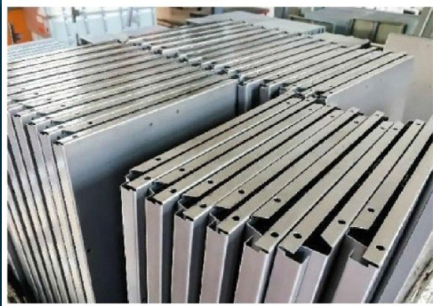
Bending of sheet metal cabinets
